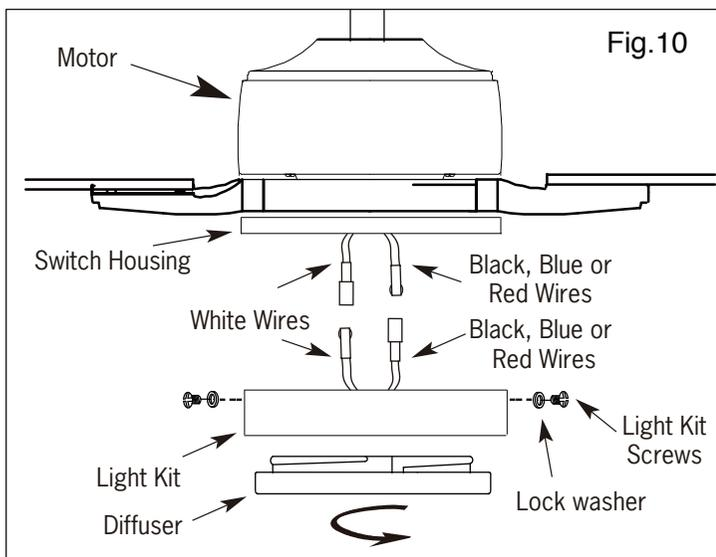
**WARNING:** Ensure that all connections, set screws and screws are securely tightened before the next step.
