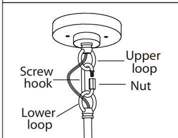
**2.** Install the length of rod that is required by threading wire through the rod and screwing it to the fixture. Screw the lower loop to the top rod.
