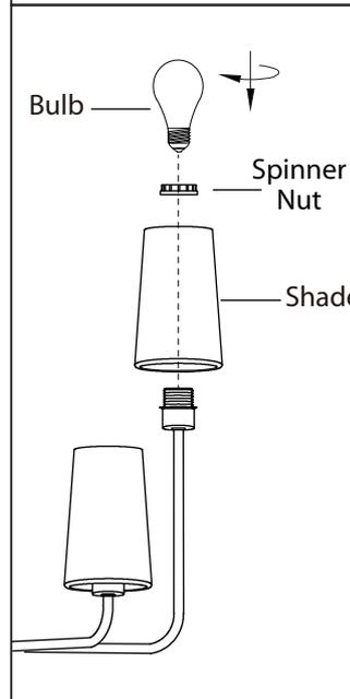
**9.** Remove spinner nut from socket. Position shade on lamp and secure with spinner nut.
