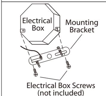
**5.** Mount the mounting bracket to electrical box using electrical box screws (not included). Make sure the studs on the mounting bracket are facing out from the electrical box.
