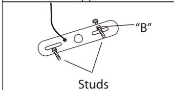
**4.** Loosen "B". Adjust stud to desired length and lock in place with "B".
