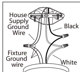
**6.** Connect the ground wires (bare copper or green) from your fixture to the ground wire (bare copper or green) or ground screw in the electrical box. Connect the black wire from the fixture to the black wire in the electrical box and connect the white wire from the fixture to the white wire in the electrical box.
