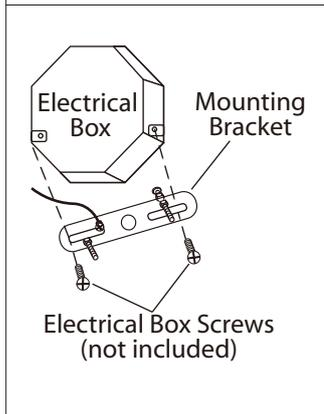
3. Mount the mounting bracket to outlet box using electrical box screws (not included). Make sure the studs on the mounting bracket are facing out from the electrical box.
