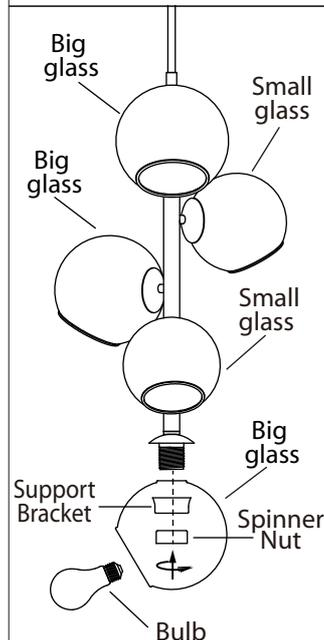
7. Remove spinner nut and support bracket from socket. Position glass on lamp and secure with spinner nut and support bracket.
