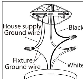
4. Connect the ground wires (bare copper or green) from your fixture to the ground wire (bare copper or green) or ground screw in the electrical box. Connect the black wire (or wire with marking) from the fixture to the black wire in the electrical box and connect the white wire from the fixture to the white wire in the electrical box.
