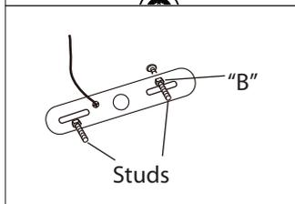
2. Loosen "B". Adjust stud to desired length and lock in place with "B".
