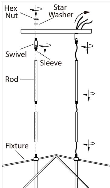
**1.** Install the length of rod that is required by threading wire through the rod and screwing it to the fixture. Install swivel to the rod, ensuring that the sleeve is at the swivel.
