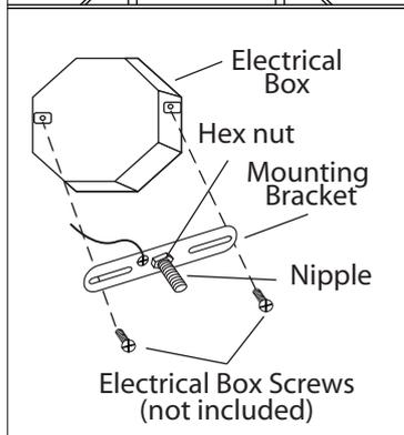
**3.** Attach nipple to mounting bracket. Adjust so it will clear hole in back of fixture and then lock nipple in place with star washer and hex nut. Attach mounting bracket to electrical box with electrical box screws (not included).
