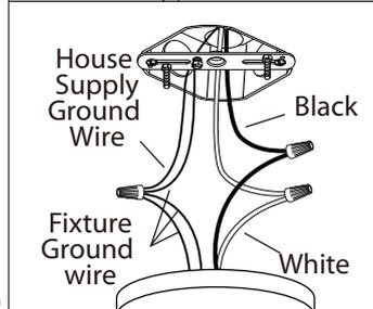
5. Connect the ground wires (bare copper or green) from your fixture to the ground wire (bare copper or green) or ground screw in the electrical box. Connect the black wire from the fixture to the black wire in the electrical box and connect the white wire from the fixture to the white wire in the electrical box.
