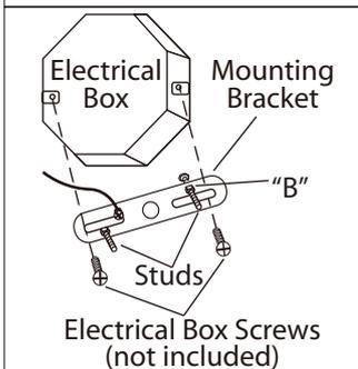
2. Loosen "B". Adjust stud to desired length and lock in place with "B".
