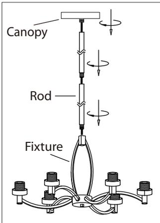
1. Install the length of rod that is required by threading wire through the rod and screwing it to the fixture. Screw the canopy to the fixture.
