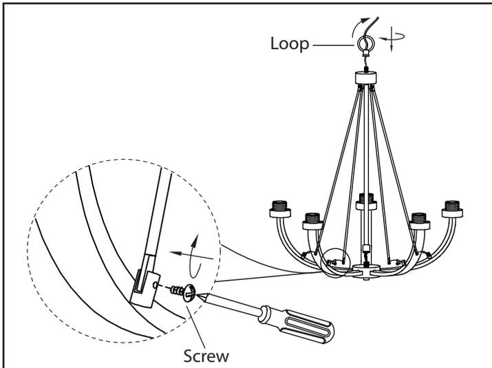
1. Tighten the loop to the stem on the fixture. Tighten the arms by the screw as shown.
