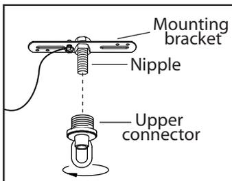
**3.** Determine the height that you would like to hang your fixture. Trim the cord and chain. Allow 10" of extra wiring for the electrical box connections.
