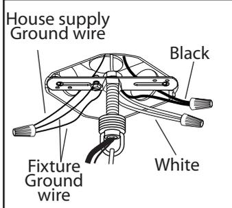
**7.** Connect the ground wires (bare copper or green) from your fixture to the ground wire (bare copper or green) or ground screw in the electrical box. Connect the black wire (or wire marked "SPT-1") from the fixture to the black wire in the electrical box and connect the white wire (or the wire with ribbed side) from the fixture to the white wire in the electrical box.
