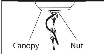
**9.** Slide the canopy up the chain and over the upper connector. Slide the nut up the chain and thread onto the upper connector.
