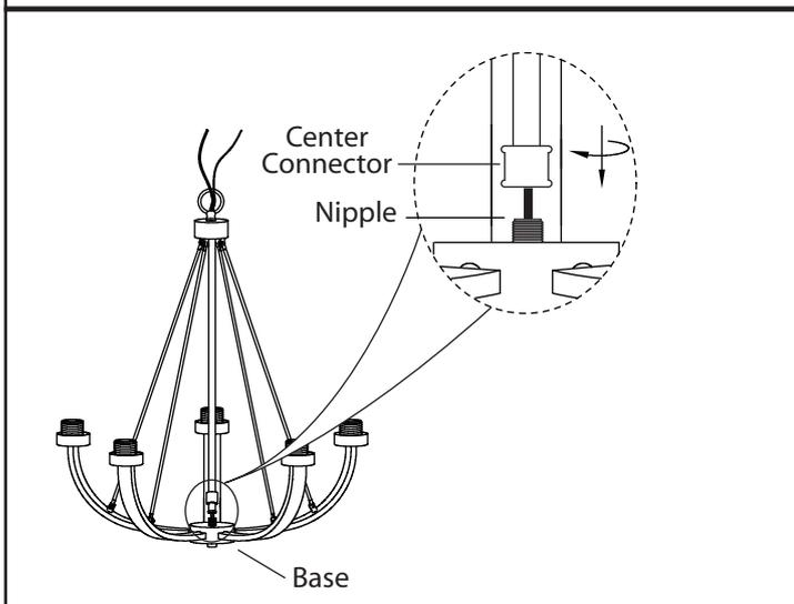
2. Pull the extra cord out from the base. Screw the center connector into the nipple.
