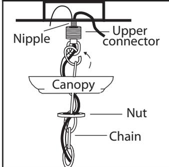
**6.** Loosen the nut on the upper connector and slide it down the chain towards the lower connector. Slide the canopy down the chain towards the lower connector. Feed the wire through nut, canopy, the upper connector and onto the nipple. Tighten the upper connector onto the nipple. Spread the other end of the chain open and fasten to the upper connector. Ensure the opening is closed.
