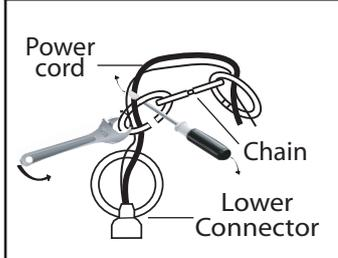
**5.** To attach chain loop to light fixture, use a screwdriver and wrench to open and close chain loop. Ensure to close the opening. Weave the power cord and ground wire through the links in the chain.
