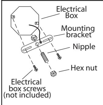
**4.** Loosen the upper connector from nipple. Attach the mounting bracket to the electrical box using electrical box screws (not included). Attach the nipple to the mounting bracket and adjust until it will clear the canopy when assembled (Place the canopy over the nipple and tighten the upper connector onto the nipple until snug. The upper connector should hold the canopy snug to the ceiling). Lock the nipple in the correct position using the hex nut.
