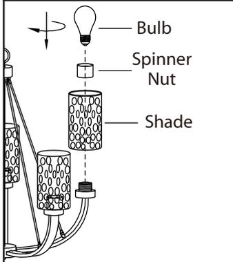
**10.** Remove spinner nut from socket. Position shade on lamp and secure with spinner nut.
