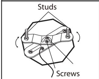
**3.** Position mounting bracket so that the fixture will be hung properly once it is mounted to the wall. Tighten the screws to hold in place.
