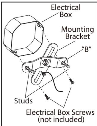
**1.** Loosen "B". Adjust stud to desired length and lock in place with "B".
