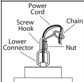
**5.** Un-Screw the screw hook and insert the lower connector into the screw hook.
