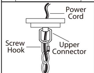
**6.** Repeat the same step for the upper connector connection. Feed the cord and ground wire through the upper loop.
