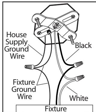
**7.** Connect the ground wires (bare copper or green) from your fixture to the ground wire (bare copper or green) or ground screw in the electrical box. Connect the black wire (or wire marked "SPT-1") from the fixture to the black wire in the electrical box and connect the white wire (or the wire with ribbed side) from the fixture to the white wire in the electrical box.
