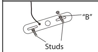
2. Loosen "B". Adjust stud to desired length and lock in place with "B".
