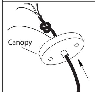
4. Adjusting the length of flexible cord. For safety, do not release the knot inside canopy.
