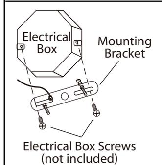
3. Mount the mounting bracket to electrical box using electrical box screws (not included). Make sure the studs on the mounting bracket are facing out from the electrical box.
