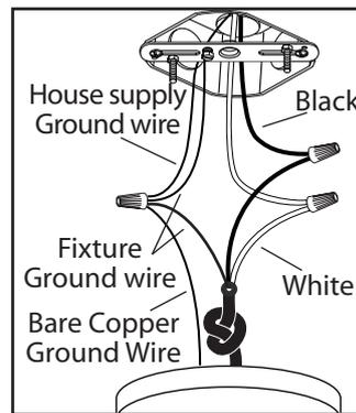
5. Connect the ground wires (bare copper or green) from your fixture to the ground wire (bare copper or green) or ground screw in the electrical box. Connect the black wire from the fixture to the black wire in the electrical box and connect the white wire from the fixture to the white wire in the electrical box.
