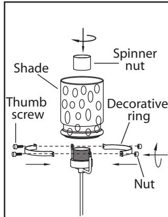
1. Turn the fixture up-side down. Remove spinner nut from socket. Position the shade on the socket. Tighten the decorative rings by thumb screws and nuts. Secure the shade with spinner nut.
