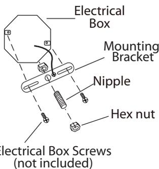
2. Loosen the upper connector from nipple. Attach the mounting bracket to the electrical box using electrical box screws. Attach the nipple to the mounting bracket and adjust until it will clear the canopy when assembled (Place the canopy over the nipple and tighten the upper connector onto the nipple until snug. The upper connector should hold the canopy snug to the ceiling). Lock the nipple in the correct position using the hex nut.
