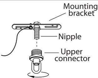
1. Determine the height that you would like to hang your fixture. Trim the cord and chain. Allow 10" of extra wiring for the electrical box connections.
