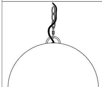
7. Slide the canopy up the chain and over the upper connector. Slide the nut up the chain and thread onto the upper connector.
