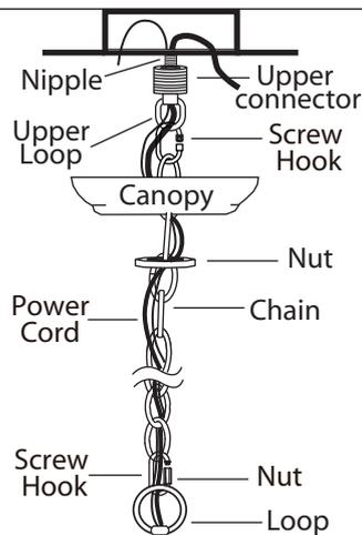
3. Connect the chain to the loop and the top loop on the upper connector using the two screw hook.
