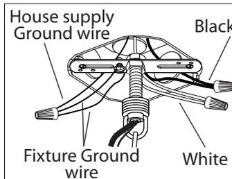
5. Connect the ground wires (bare copper or green) from the fixture to the ground wire (bare copper or green) or ground screw in the electrical box. Connect the black wire (or wire marked "SPT-1") from fixture to the black wire in the electrical box and connect the white wire (or the wire with ribbed side) from fixture to the white wire in the electrical box.
