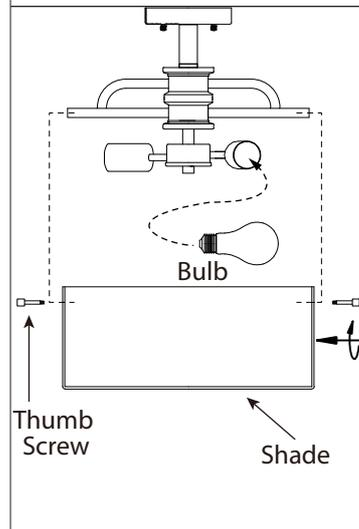
7. Install specified bulb type and wattage (not included).
