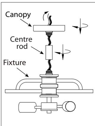
1. Screw the centre rod and canopy to the fixture.
