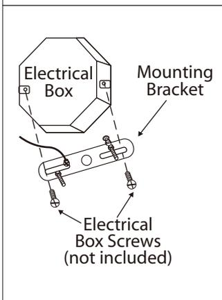
3. Mount the mounting bracket to electrical box using electrical box screws (not included). Make sure the studs on the mounting bracket are facing out from the electrical box.
