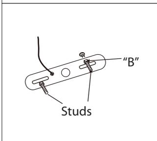
2. Loosen "B". Adjust stud to desired length and lock in place with "B"
