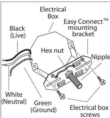
**1.** Attach nipple to mounting bracket. Adjust so it will clear hole in back of fixture and then lock nipple in place with hex nut. Attach mounting bracket to electrical box with electrical box screws (not included).
