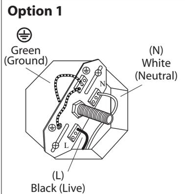
**2. Option 1:** Connect (push) electrical wires from electric box (house wiring) into correct inserts.
