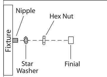
**4.** Once connections of wires are completed, carefully tuck wires and wire nuts into the electrical box making sure no bare wire (on the black and white) is visible at the wire nuts. Secure the fixture to the nipple tightening by star washer and hex nut. Screw the finial to the nipple.
