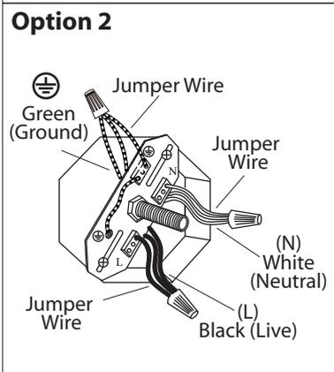
**Option 2:** For multiple green (ground), black (live) and white (neutral) wires joined in the electrical box (house wiring), attach a single "green," "black" and "white" jumper wire before connecting. Strip 7mm from a 6 in. jumper wires supplied. Then connect (push) wires into the correct inserts.
