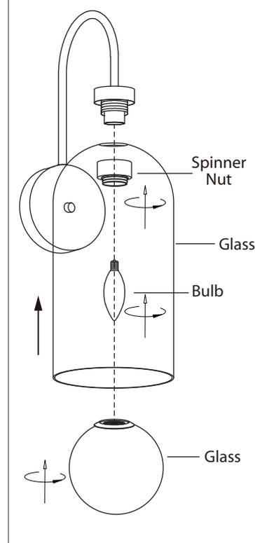
**5.** Remove spinner nut from socket. Position glass on lamp and secure with spinner nut. **(Please check the glass before installing for any cracks. Do not overtighten the spinner nut to attach the glass to the fixture.)**
