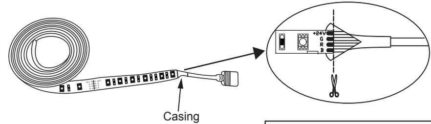
2. CONNECT—use the connector to connect the strip. Insert the end of the strip and make sure the flat welding plate is well inserted into the connector.
