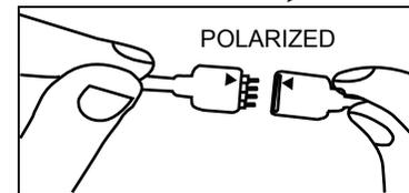
CONNECT – Ensure the plug is polarized. Connect the power feed cable assembled on the tape to the RGB Dimmer Control.
