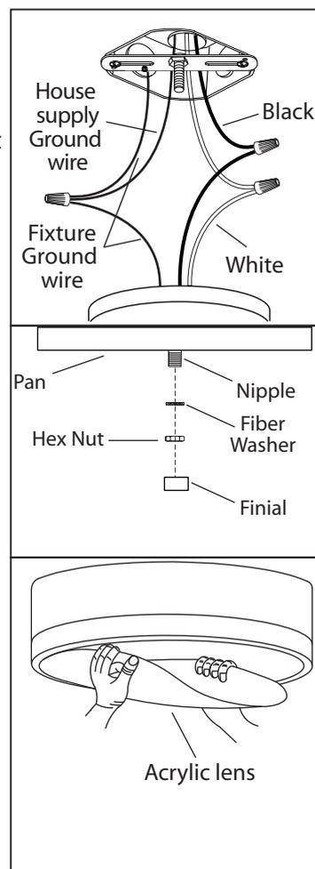
3. Connect the ground wires (bare copper or green) from your fixture to the ground wire (bare copper or green) or ground screw in the electrical box. Attach the black wire from the light fixture to the black wire in the electrical box. Attach the white wire from the light fixture to the white wire in the electrical box.
