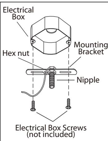
1. Attach nipple to mounting bracket. Adjust so it will clear hole in back of fixture and then lock nipple in place with hex nut. Mount the mounting bracket to electrical box using electrical box screws (not included).
