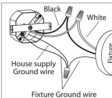
3. Connect the ground wires (bare copper or green) from your fixture to the ground wire (bare copper or green) or ground screw in the electrical box. Attach the black wire from the light fixture to the black wire in the electrical box. Attach the white wire from the light fixture to the white wire in the electrical box.
