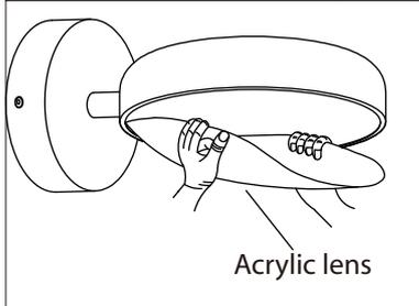
6. Squeeze gently and insert the acrylic lens as shown.
