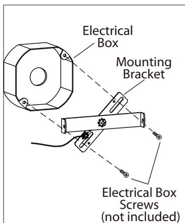
1. Mount the mounting bracket to electrical box using electrical box screws (not included).
