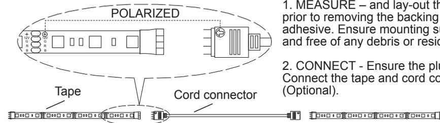
1. MEASURE – and lay-out the installation prior to removing the backing exposing the adhesive. Ensure mounting surface is clean and free of any debris or residue.
