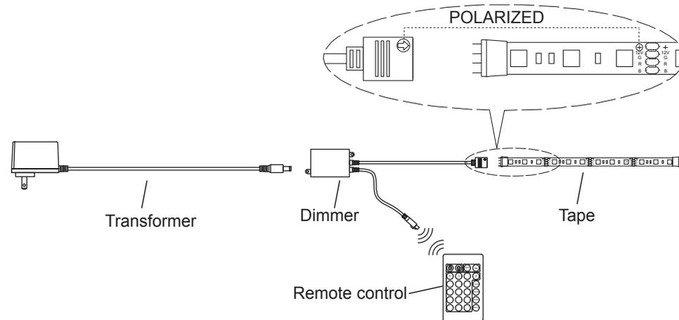
4. CONNECT – Connect the tape to the dimmer. Then connect the dimmer to the transformer and plug in. The dimmer must be placed in a dry location. Use the two screws to hold the dimmer in place.
