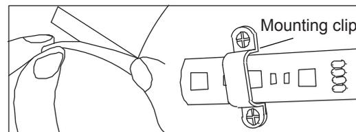
3. MOUNT – Remove the backing to expose adhesive tape. Place in the desired location. To obtain optimum adhesion, ensure the surface is clean. Mounting clips are also provided for extra support with screws.
