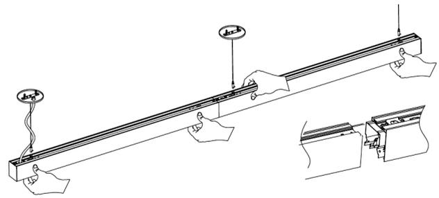
**Note:** Since **18 AWG** wires are used in these luminaires, the max current allowable is **6A**. Please refer to your local electrical code to determine the maximum luminaire allowed on a power line.
