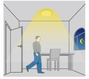
With insufficient ambient brightness, the light dims to 100% when motion detected
