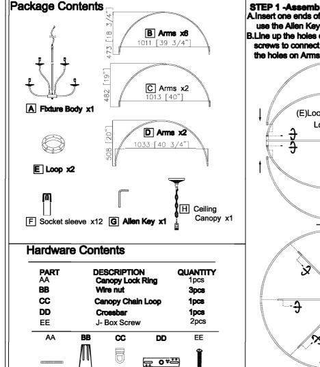
STEP 1 -Assemble the Bird Case and the Fixture Body.
