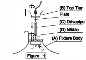
STEP 2 Install the Canopy Chain Loop and Nipple
