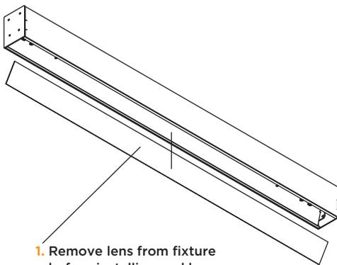
1. Remove lens from fixture before installing and keep in a safe place.
