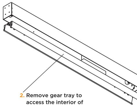
2. Remove gear tray to access the interior of the enclosure.
