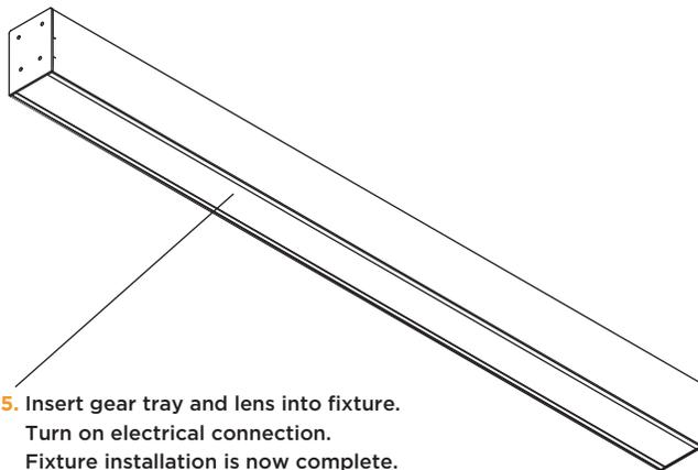
5. Insert gear tray and lens into fixture.
