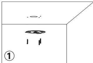
1. Disconnect electrical power and fix the bracket on the J-box.
