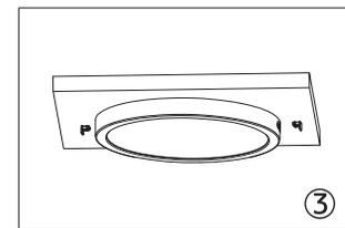
3. Fixing the lamp body on bracket and fix tightly
