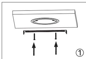
1. Fixing bracket on terminal box
