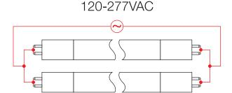
NOTE: Both pins on each end of lamp must be connected to line voltage as shown above. If lamp holder is a "non-shunted" (T12) type, it must be shunted (shorted) by external jumper. Most T8 lamp holders are internally shunted and will not require an external jumper.
