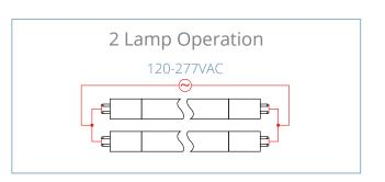
Note: both pins must be connected.
