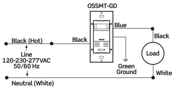
**Note:** Ground wire must be connected.
