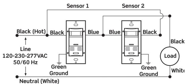
**Note:** Ground wire must be connected.
