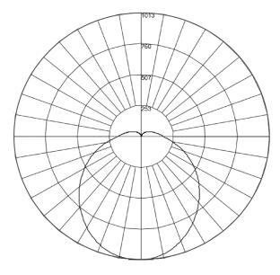
Maximum Candela = 1013.4 Located at Horizontal Angle = 150, Vertical Angle = 4 Vertical Plane through Horizontal Angles (0 - 180)
