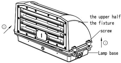
**1** Use a screwdriver to unscrew the lamp screws and remove the upper half of the fixture.
