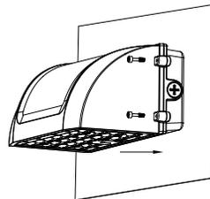
**8** Use screws to lock the fixture. Installation completed.
