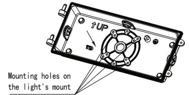
**3** Unscrew the cover of the entry hole on the lamp base and remove the cover.
