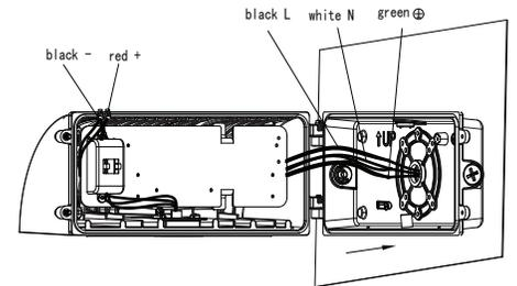
**6** Connect the input wire and the dimming wire of the light, then put the connected wires into the embedded terminal box.
