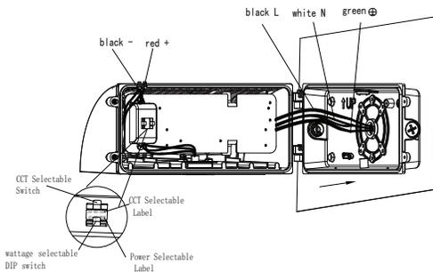
**7** After the wiring completed, set the CCT and power value through the internal switches. According to the label, users can dial the desired color temperature value and power value.
