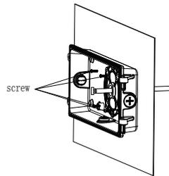
**5** Use screw to lock the lamp base on the embedded junction box.
