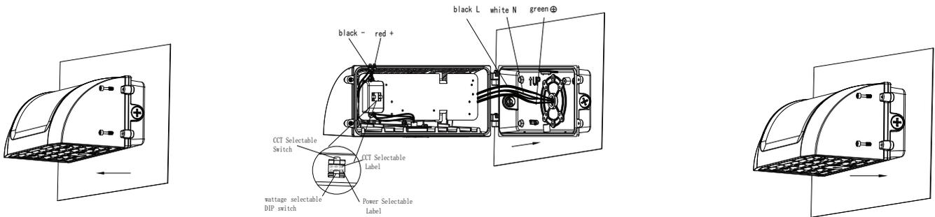
**1** Use a screwdriver to unscrew the lamp screws and remove the upper half of the fixture.
