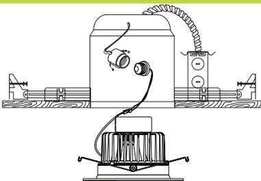
Socket adapter removes from module, allowing installation to be quick and easy. Simply screw in the adapter and plug in the module. Turning off the entire module is not required.
