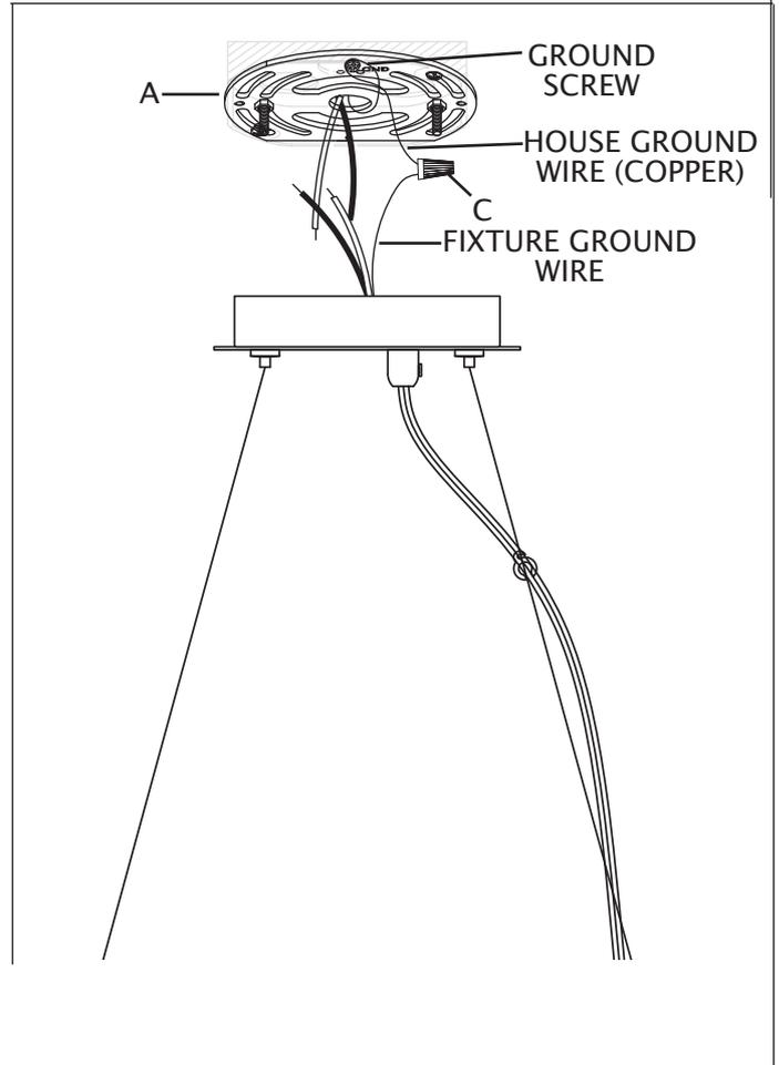
16. Twist end of house lead wire (black) and end of fixture lead wire together. Twist wire nut (C) onto ends of wires. Completely tighten wire nut (C). Twist end of house neutral wire (white) and end of fixture neutral wire together. Twist wire nut (C) onto ends of wires. Completely tighten wire nut (C). Reference chart to the right for correct wire connections.
