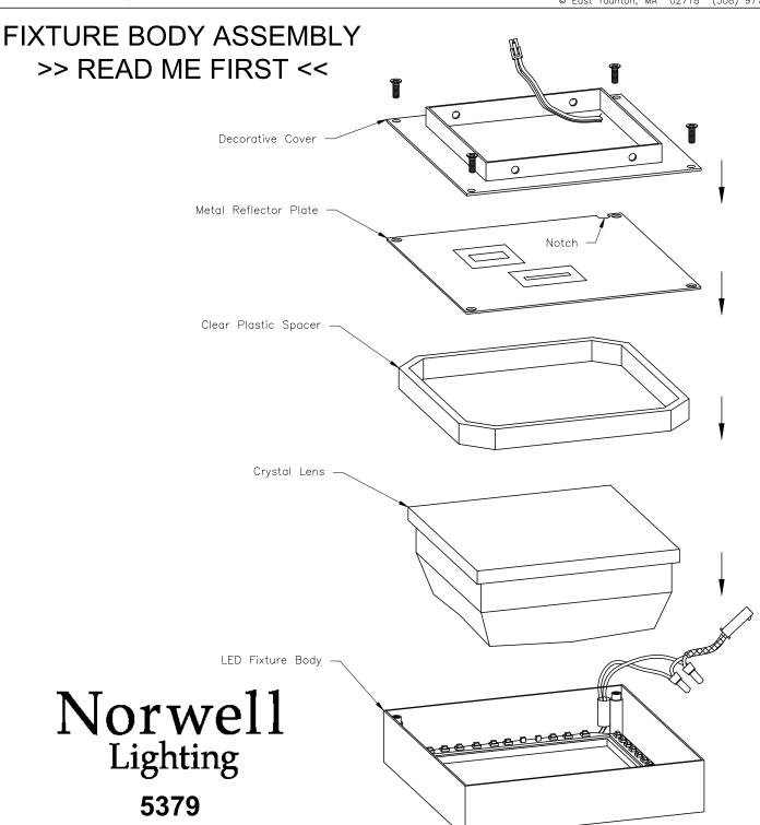
NOTE: to protect the Crystal Lens from possible damage during shipping, this fixture ships partially disassembled.
