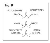
\*Note: If your fixture has a sliding backplate loosen the set-screw and slide the backplate toward the socket (be careful not to scratch the finish). Mount the fixture to the box and wire the fixture as described in section B. When finished, slide the backplate against the wall and tighten the set-screw.
