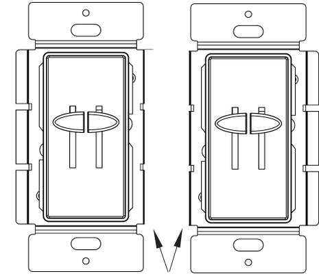
Tabs Removed for Multigang installation
