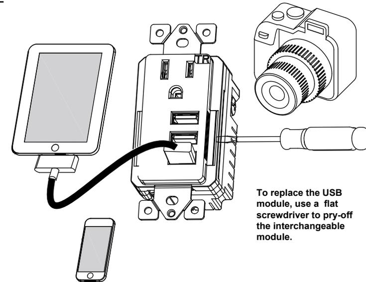
**To replace the USB module, use a flat screwdriver to pry-off the interchangeable module.**
