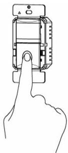
**OCCupancy position:** When the ambient light level is reached, the Load will automatically turn ON when motion is detected and automatically turn OFF when the selected time delay has expired.
