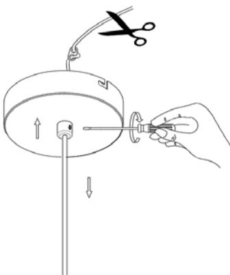
Before installation to ceiling,adjust fixtures to desired length.
