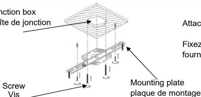
Attach the mounting plate to junction box with screws provided.
