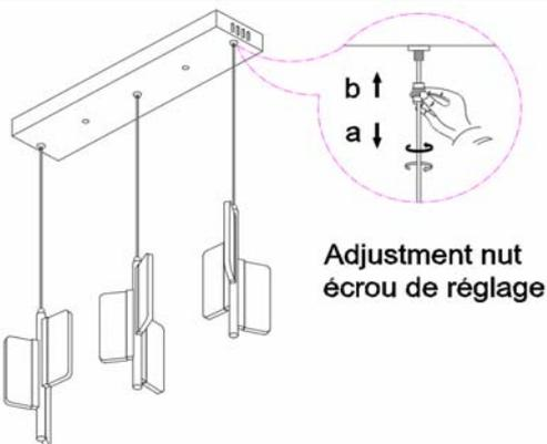
Before installation to ceiling,adjust fixtures to desired length by pushing wire up into canopy,then coiling up excess wire, minor adjustment can be made after installation.To lower or lengthen wire,depress button sleeve located where wire comes out of canopy.
