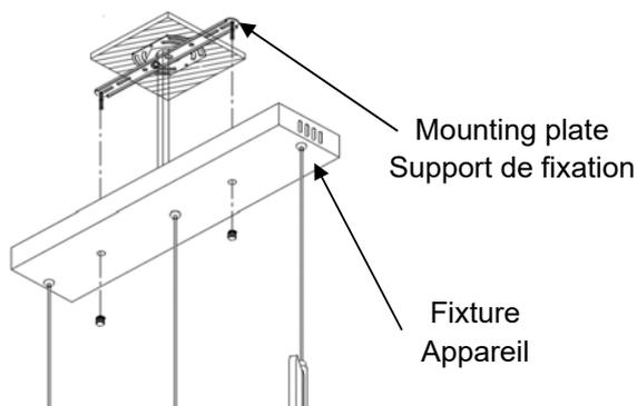
Attach the fixture to the mounting plate with cap nuts provided.
