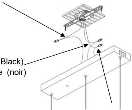
Connect the GROUND WIRE from junction box to GROUND (COPPER or GREEN) wire from fixture with a wire nut. Connect the NEUTRAL WIRE from junction box to NEUTRAL (WHITE) wire from fixture with a wire nut. Connect the LINE WIRE from junction box to LINE (BLACK) wire from fixture with a wire nut.
