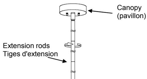
Connect extension rods to desired length and feed wires through rods and canopy.
