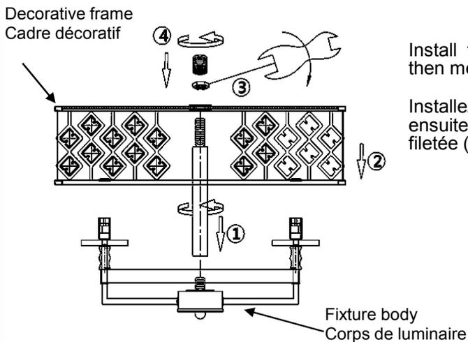
Install the metal rod to fixture body (1), then decorative frame(2), then metal washer(3), then nipple(4).
