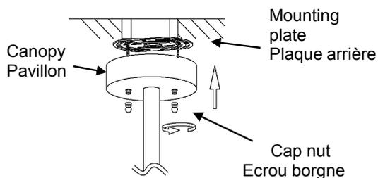
Install the canopy to mounting plate with cap nut provided.
