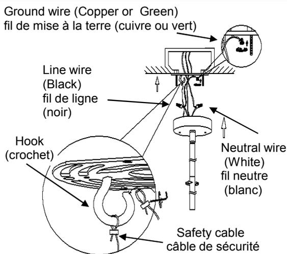
Secure the safety cable to the hook on mounting plate. Connect the GROUND WIRE(Green or Copper) from junction box to GROUND WIRE(Labeled) from fixture by using a wire nut. Connect the NEUTRAL WIRE(White wire) from junction box to NEUTRAL WIRE(White wire) from fixture with a wire nut. Connect the LINE WIRE(Black wire) from junction box to LINE WIRE(Black wire) from fixture with a wire nut.
