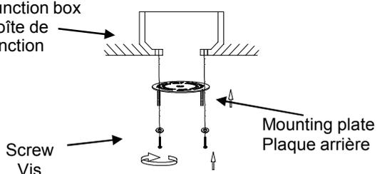
Attach the mounting plate to junction box with screws.
