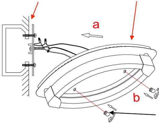
Attach fixture to mounting plate with cap nuts provided.
