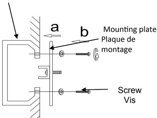
Attach mounting plate to junction box with screws provided.
