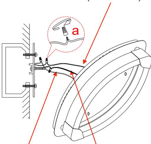
Connect the GROUND WIRE from junction box to GROUND (or GREEN) with a wire nut. Connect the NEUTRAL WIRE from junction box to NEUTRAL (WHITE) wire from fixture with a wire nut. Connect the LINE WIRE from junction box to LINE (BLACK) wire from fixture with a wire nut.
