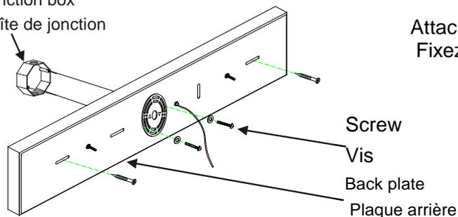
Attach the back plate to the junction box.
