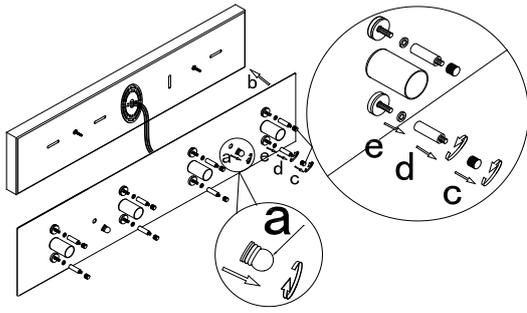
a. Attach the face plate to the back plate with cap nuts provided.
