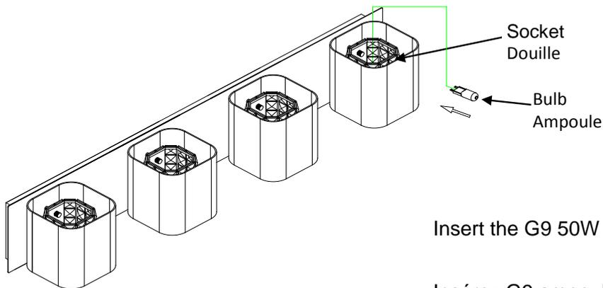
Insert the G9 50W Bulb to the socket
