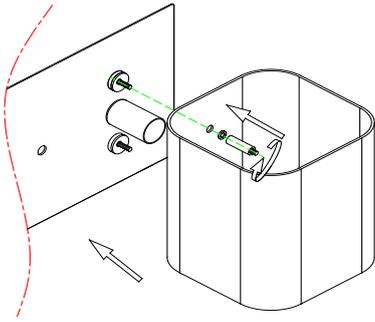
Install the glass shade and rubber washer to the face plate.
