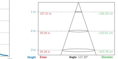
Note: The curves indicate the illuminated area and the average illumination when the luminaire is at a different distance.
