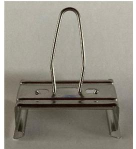
3. CABLE MOUNTING (Cable Mounts are not included): Secure the mounting cables to the mounting surface at the desired location and height. Attach the mounting cables to the stainless-steel mounting brackets and snap the mounting brackets onto the back of the fixture. The brackets will snap onto the back of the fixture at any location inside the end caps.
