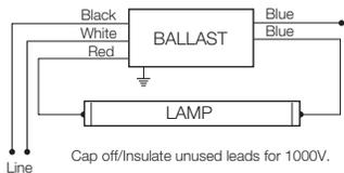
Note: For one lamp application, cap blue lead. Insulate to 1000 volts.
