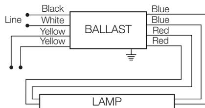
Note: For one lamp application, individually cap each yellow lead. Insulate to 600 volts.
