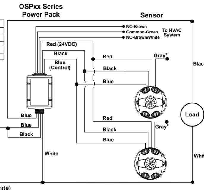
**\*NOTE:** When using the Photocell function, connect the Gray wire of the sensor to the Blue wire of the power pack. **DO NOT** use the Blue wire of sensor.
