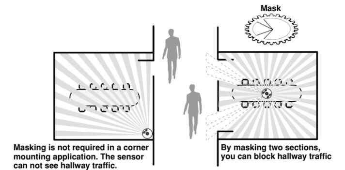
Masking is not required in a corner mounting application. The sensor can not see hallway traffic.
