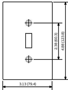
Note: Add 1.81" (46.0mm) for each additional gang. Midway wallplates can be mounted onto larger-volume outlet boxes and/or used to hide wall irregularities. Midway wallplates are a full 0.375" taller and wider than standard size wallplates.
