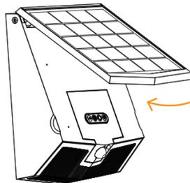
adjust solar panel angle to maximize sunlight & allow snow to slide off
