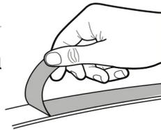
2. Press LED tape firmly onto clean smooth surface that adsorbs heat, such as metal or glass. Start at one end and gradually move along surface, making sure tape is smooth and not creased.
