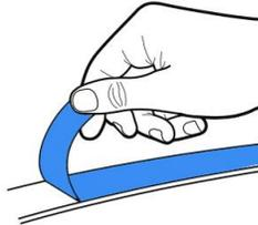
2. Press LED tape firmly onto clean smooth surface that adsorbs heat, such as metal or glass. Start at one end and gradually move along surface, making sure tape is smooth and not creased
