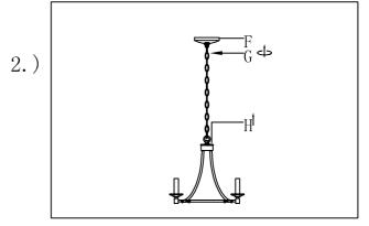
Step. 2: Attach appropriate amount of chain to loop to achieve desired mounting height. Thread wire through every 3rd loop of chain.
