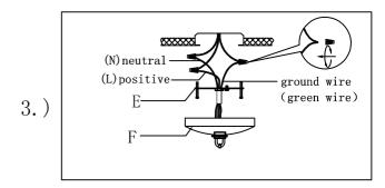
Step. 3: Wire fixture to wires in outlet box. Copper/Green wire is for Ground.
