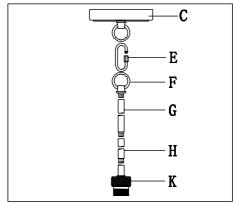
Step.1: Run wire through stems and combine stem lengths to loop, locked the hook with top and
