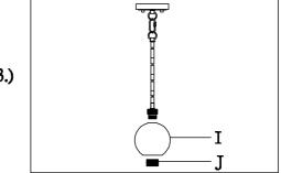
Step3: Attached the Glass(I) to the socket, then secured by socket ring(J)
