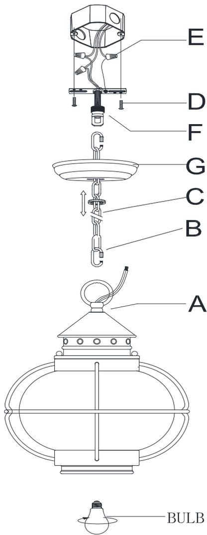
1. Attach appropriate amount of chain to loop to achieve desired mounting height. Thread Copper wire and SPT wire through every 3rd loop of chain.
